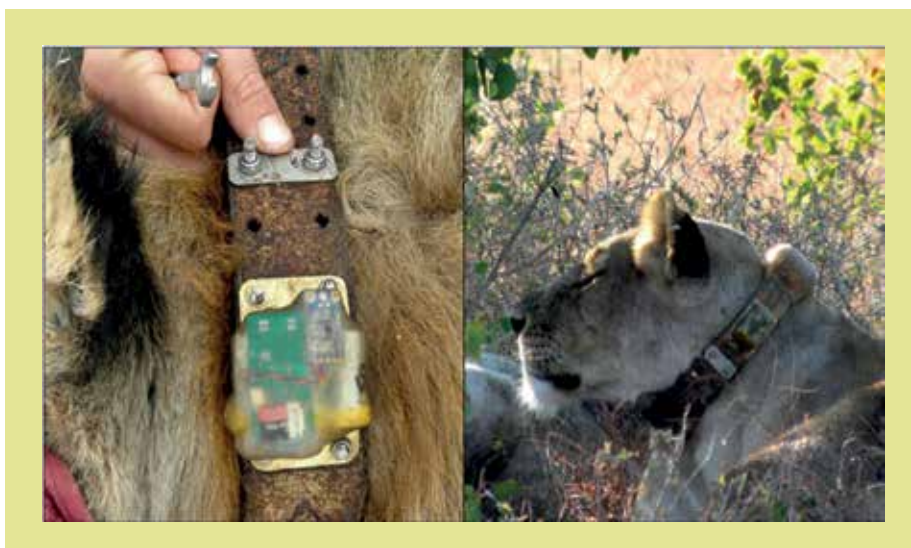
Figure 1. [left] Acoustic bio-logger attached to GPS collar on a lioness.
